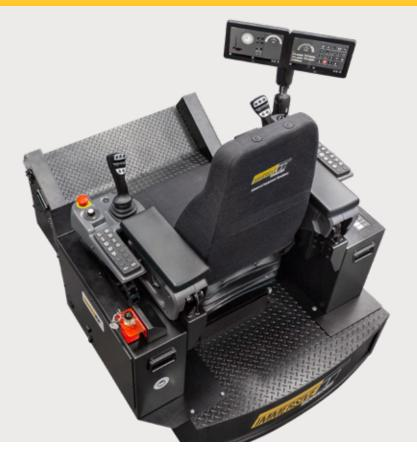
Simulated main and secondary displays including interlocks, drilling, levelling and propelling dashboards
