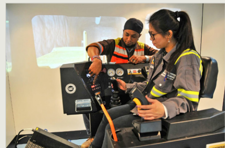
Trainee at PT Freeport Indonesia on an Immersive Technologies IM360 simulator with LHD R1600G Conversion Kit®
