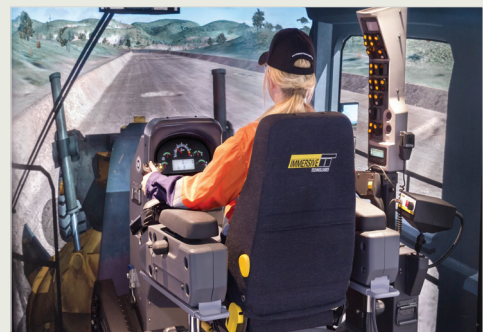
Immersive Technologies' new simulator module includes a complete replica cab of the Caterpillar 24M Motor Grader, with fully functional controls and instrumentation sourced directly from Caterpillar. The combination dash mounted instrument cluster and the CAT Advisor Messaging System provide key machine operating information and give the operator insight into the machine's operation and maintenance needs.
